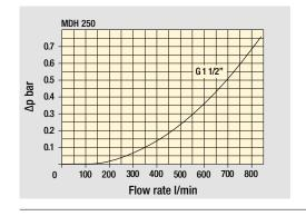
Bypass valve pressure drop
