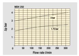
The curves are plotted using mineral oil with density of 0.86 kg/dm³ in compliance with ISO 3968. Δp varies proportionally with density.
