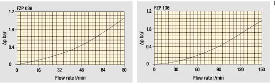
The curves are plotted using mineral oil with density of 0.86 kg/dm<sup>3</sup> in compliance with ISO 3968. Δp varies proportionally with density.
