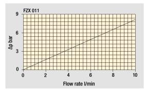
The curves are plotted using mineral oil with density of 0.86 kg/dm³ in compliance with ISO 3968. ∆p varies proportionally with density.
